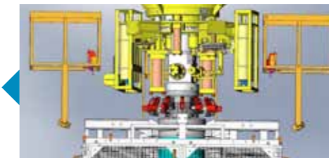
860mm Nose extension, cranked torque reaction & 2,000 N·m tool for long reach Wellhead connectors
