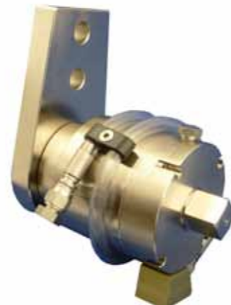
2,000 N·m 15:1, no grease, with pressure compensation, for ROV sub-sea use
