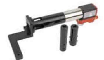
PT-72 fitted with special valve mounting & drive adaptors
