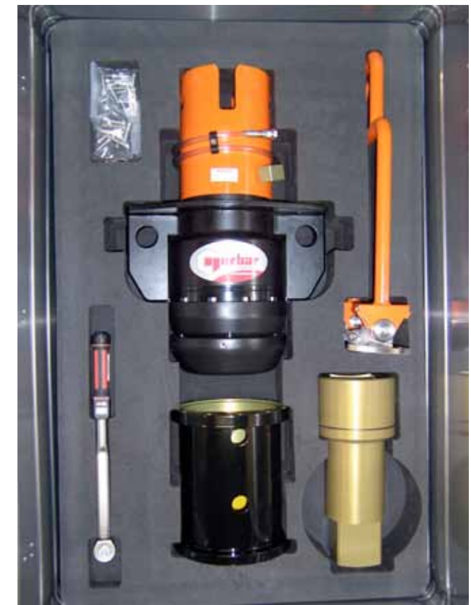
API 17D 4-6/4-7/4-7 short interchangeable kit 34,000 N·m
