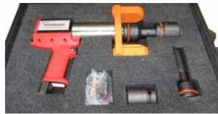
API Class 2 & 3 reaction kits for valve run-down with hand held tool. See valve testing sheet for full testing kits
